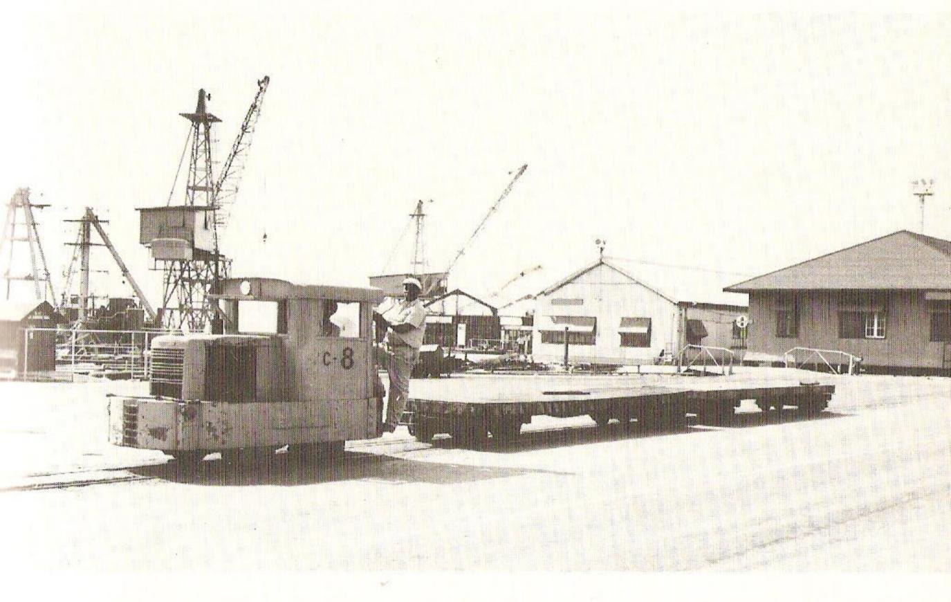
One of Lago's fleet of 11 6-ton Brookville locomotives on the 'main line' along the main refinery road. All of Lago's locomotives were numbered with the prefix 'C' to designate them as locomotives. The flatcars have  $4 \times 12$  ft. decks, and 12-inch cast steel wheels, made by the Gregg Cast Metal Co. The cars were coupled with link and pin couplers, the coupler bolsters swiveling with the trucks to give greater turning capacity.
